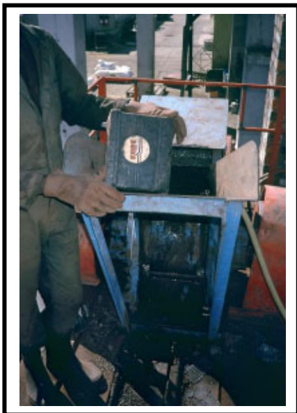
Fig. 3: Hammer mill crushing whole Batteries
