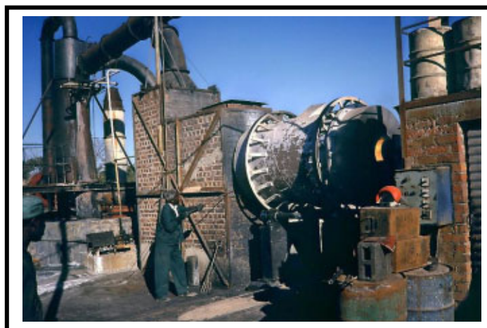
Fig. 5: Rotary drum furnace for battery scrap recycling
