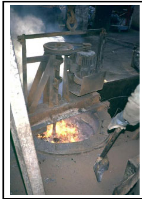
Fig. 6: Refining of crude lead in a kettle
