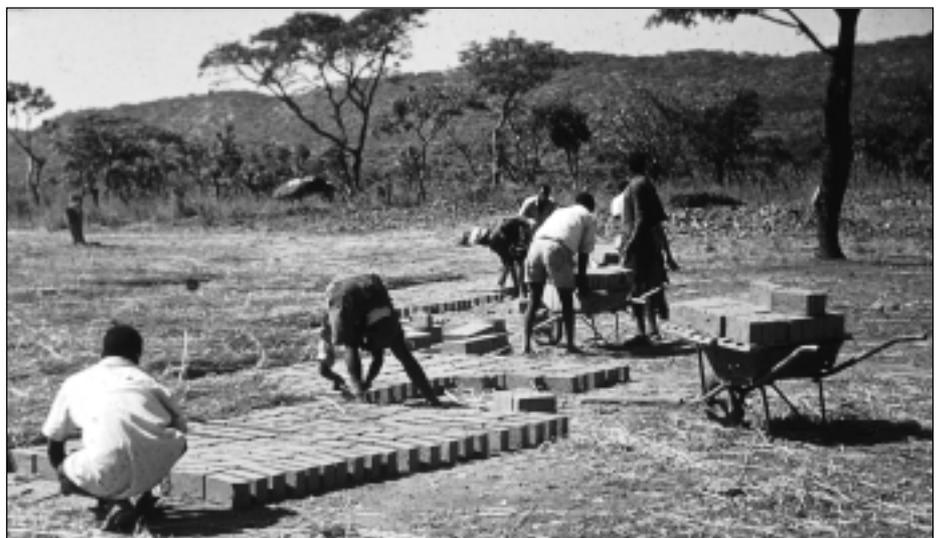
Fig. 7: Bricks are taken by wheelbarrow to the drying ground and turned on edge, covered with grass
