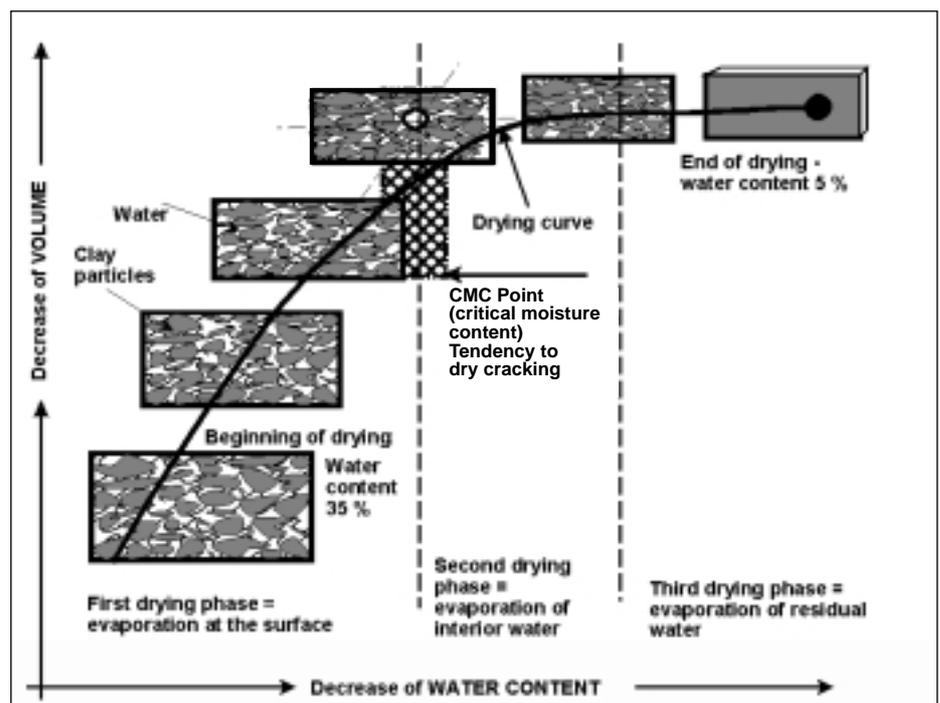
Fig. 2: Schematic drawing of drying in three phases
