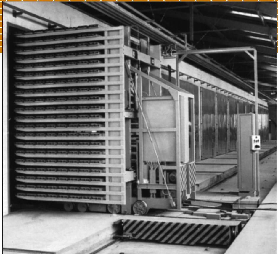
Fig. 10a: Chamber dryer for roofing tiles: automatic conveying system with finger and transfer car operation
