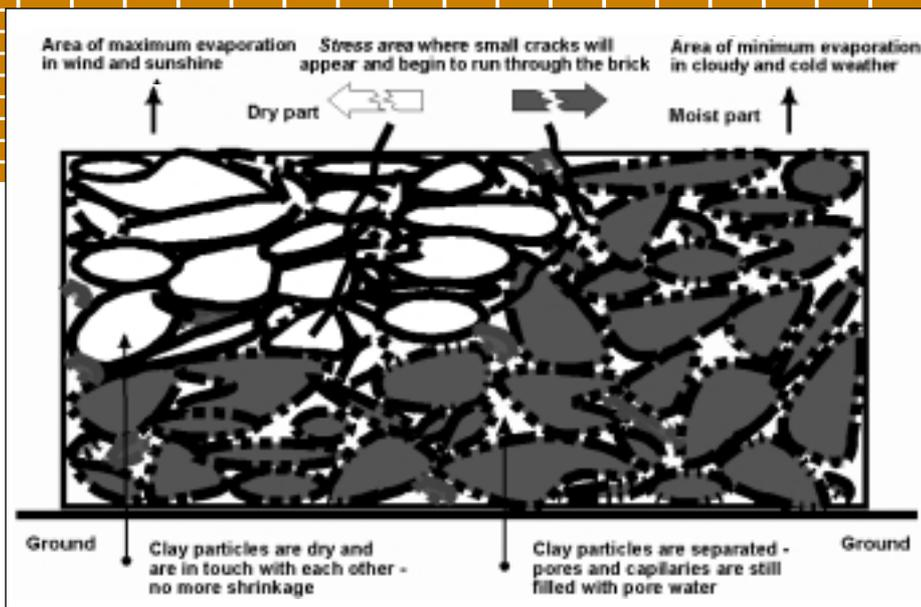
Fig. 3: Schematic drawing of "unbalanced" drying
