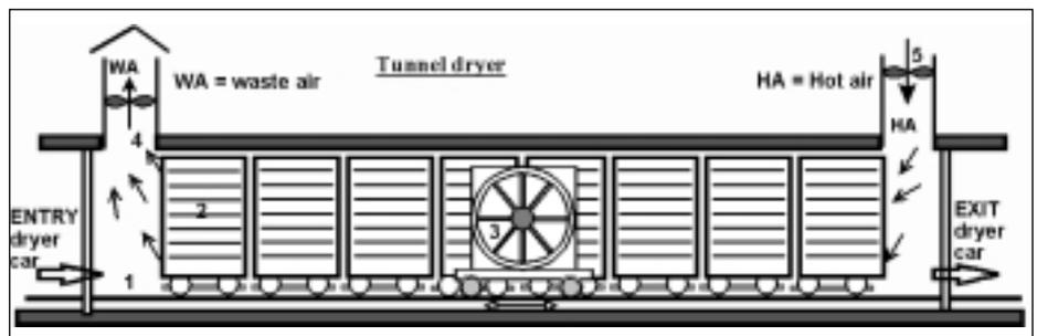
Fig. 11: Schematic drawing of artificial dryer: tunnel dryer with drying charge pushed on dryer cars through horizontal air flow
