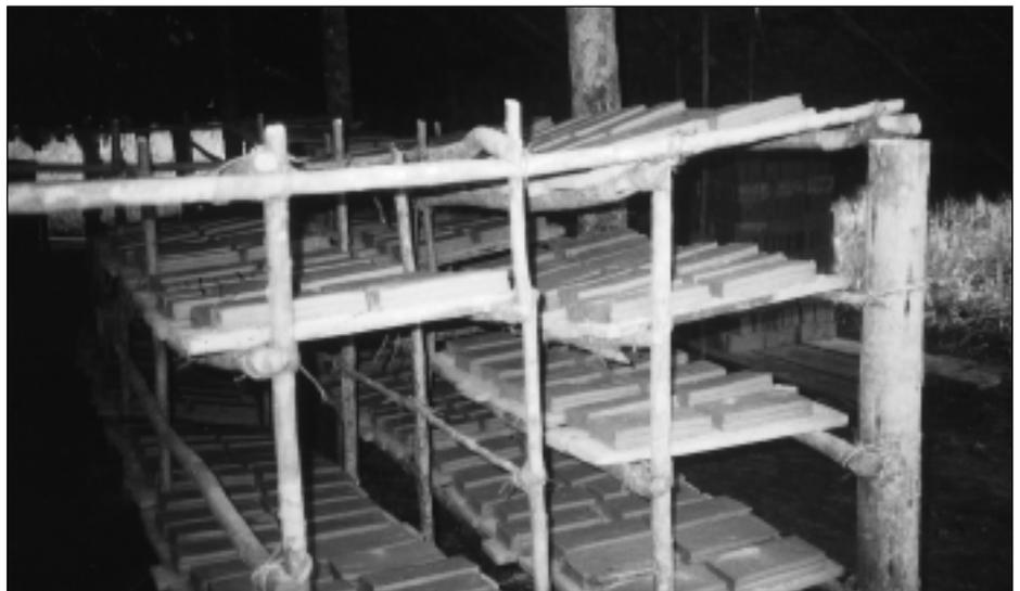
Fig. 6: Simple method of drying floor tiles on racks under a grass roof
