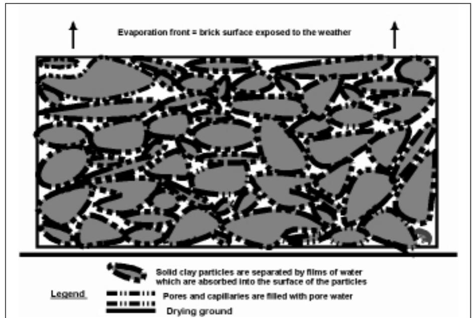
Fig. 1: Schematic drawing of clay particles enveloped in a moisture film surrounded by pores and capillaries
