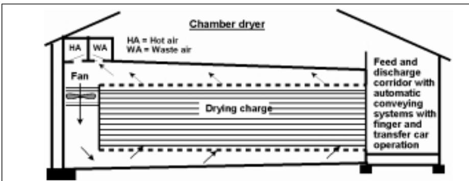
Fig. 10: Schematic drawing of artificial drying: chamber dryer with vertical air flow and with drying charge staying idle
