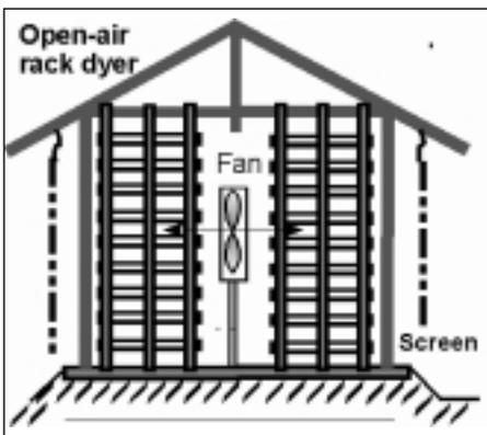
Fig. 9: Schematic drawing of natural drying: rack drying under cover
