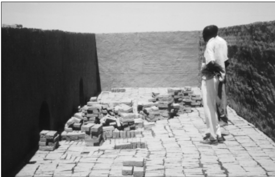
Fig 5: Stacking bricks for firing in a permanent brick clamp in Sudan.
